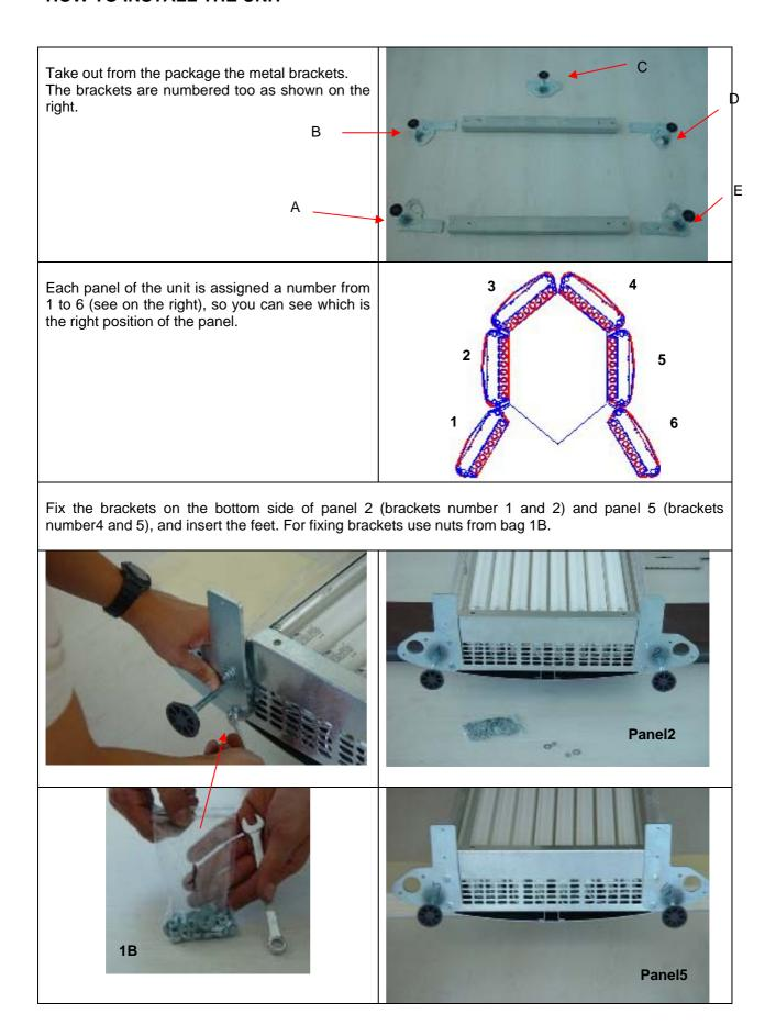
Insert the 2 long metal brackets on panel 2, then fix them with screws in bag 1A (see below); <u>Do not attach all at this time.</u>
